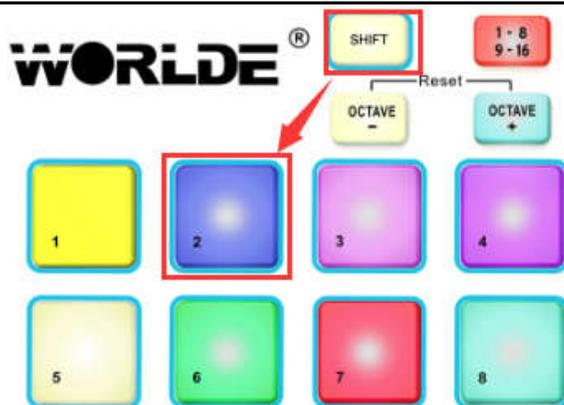
In the picture above the combination of the Shift button and Pad 2 will select Preset #2 from the TUNAMINI preset memory locations.
