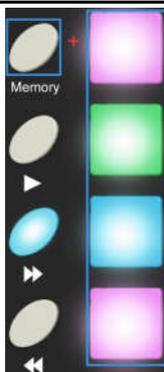
In the picture above the combination of the Memory button and Pad 2 will select Preset #2 from the ORCA PAD 48 preset memory locations.
